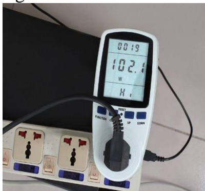
Fig. 3. Preliminary cluster evaluation: 1 – wattmeter for P_j = f_j(CPU_j) defining; 2 - P_j = f_j(CPU_j) functions got experimentally.
